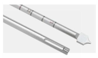
The included TightRope drill pin features a 4 mm spade tip and a closed eyelet with suture recesses for easy passage. The shaft diameter is 2.4 mm. The pin features laser markings in 5mm increments up to 20 cm. The laser marking are calibrated off the trailing edge of spade tip (a.) (Hook the back of the spade on the cortex to measure). The overall pin length 406 mm (16 in).
